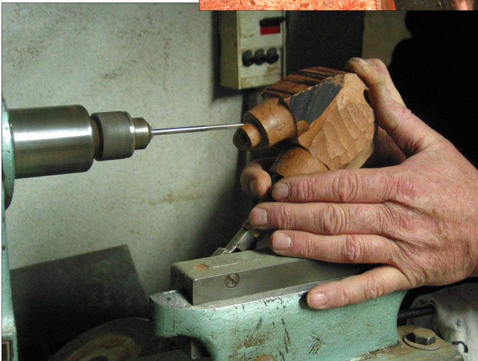
Drilling of the draft hole
